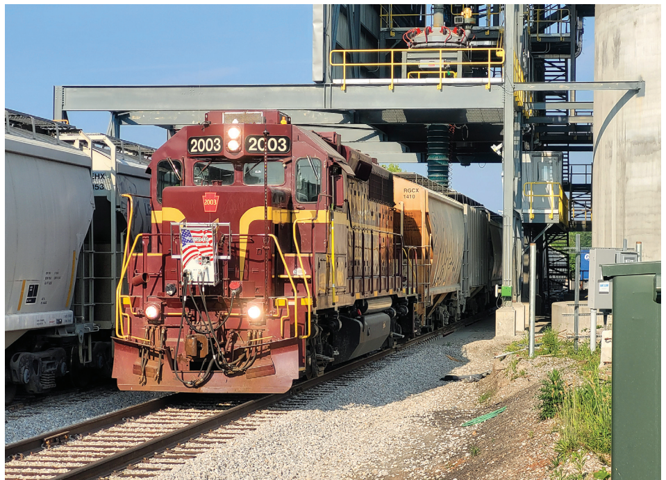
LIRC crews handle remote-controlled in-plant indexing operations for Heidelberg.
